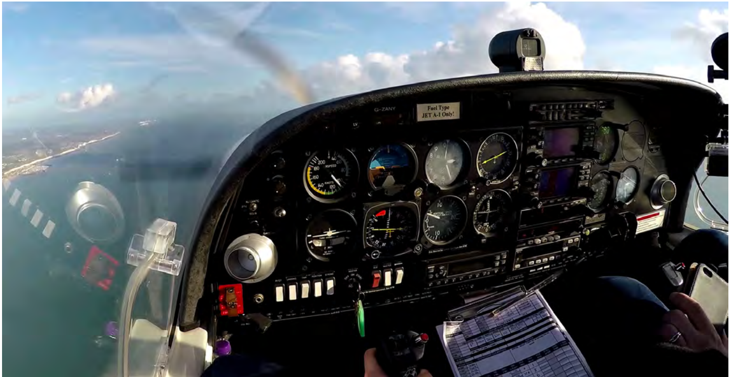
Above Panel of the Diamond DA40 with the original 'steam' gauge instruments
