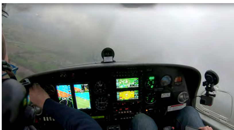
Top Panel upgraded with Aspen primary and multi-function displays, centre, and Garmin GTN 650 Xi navcomms
